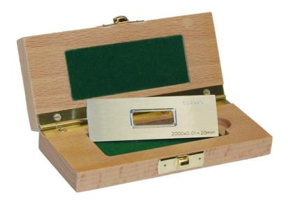
The scale is produced as a vacuum deposited chrome image on a glass disc, with a cover-glass cemented on top. This is mounted in a stainless-steel slide mount and is supplied in a polished wooden case. Internationally traceable certificates of calibration are available to satisfy the requirements of ISO.
